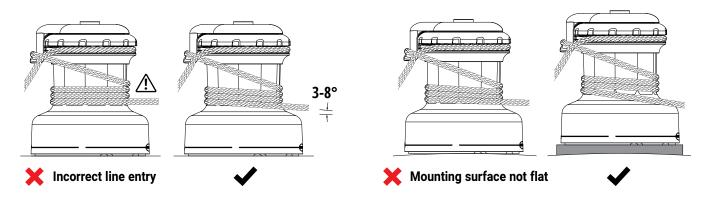
The drive gear should be aligned to the line entry as per the diagram and as indicated on the drilling template.
