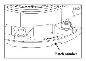
To assist with any future service inquiries, your winch has a batch number that is stamped onto the base of the centre stem in the location shown below. The self-tailing arm and drum need to be removed to access the batch number.
