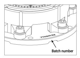
To assist with any future service inquiries, your winch has a batch number that is stamped onto the base of the centre stem in the location shown below. The self-tailing arm and drum need to be removed to access the batch number.
