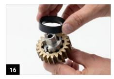
Malfunctioning pawls may lead to unexpected release of the winch force resulting in serious injury to the user and others. Check the functioning of each pawl by depressing against the spring. The pawls should move smoothly, and automatically return to their normal position to engage within the gears. If the pawls do not work correctly replace the springs and check again.
