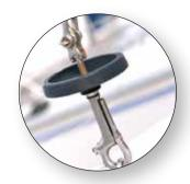
For fitting a jib, setting up a genoa or a solent jib... Both for safety and performance reasons, fitting a removable inner forestay is strongly recommended when there is a roller furling system. Wichard offers a whole range of babystay adjusters.
