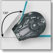
For a 120° angle: The load factor will be 180%. A load of 100 Kg on the line will represent a load of 180 Kg on the block.
