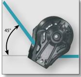
For a 45° angle: The load factor will be 75%. A load of 100 Kg on the line will represent a load of 75 Kg on the block
